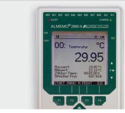
ALMEMO<sup>®</sup> precision measuring instrument with data logger function. Comprehensive range of functions for all application areas. Increased measuring accuracy, fast measuring rate. Generously dimensioned graphics display, bright illumination. 9 measuring inputs Runs on rechargeable batteries, charging via the device itself
