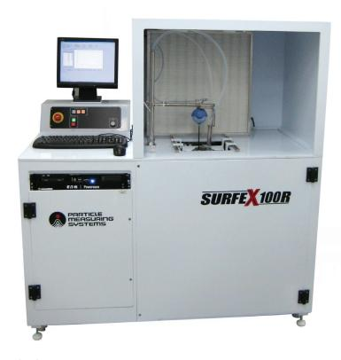
Surfex from Particle Measuring Systems is a completely integrated testing station designed to measure particle levels on almost any type of complex shaped part. The Surfex combines ultrasonic extraction, particle measurement, high-purity fluidics, and automated software control to reduce testing time and therefore reduce the cost of parts testing. A wide range of options customizes the Surfex for your application.
