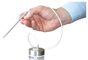
monitored. The body of the data recorder can be kept in another location. The rigid 4" probe houses an RTD temperature sensor which provides fast response time and accurate readings. Each reading is date and time stamped.
