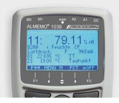
Reference measuring instrument for humidity High-precision measuring with Pt100 psychrometer Resolution Temperature 0.001 K Relative humidity 0.01 % Dew point 0.01 K
